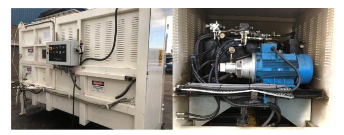
3 Phase , Heavy Duty, Blade Compactor Heads. These Stationary units are designed to be chute fed through the top of each compactor head. Each unit is supplied with "Bolt Down" bin rails, a compactor mounted control panel and soft start plc controls.
